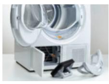
EcoDry technology consists of a perfectly working filtration system and a maintenence-free heat exchanger. This system ensures that fluff does not clog up the heat exchanger. With systems without EcoDry the heat exchanger can clog up over time, which results in constantly increasing energy consumption and longer drying times throughout the life cycle of the tumble dryer.
